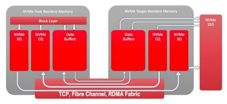
Figure 2 -- NVMe-oF with Current Fabrics
