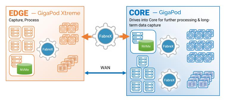
The diagram above shows at left the ruggedized GigaPod Xtreme, which can be deployed at the edge, and at right a GigaPod, located in the core datacenter. The unique value of GigalO's FabreX dynamic memory fabric is the ability to combine these into one seamless and dynamic environment.
