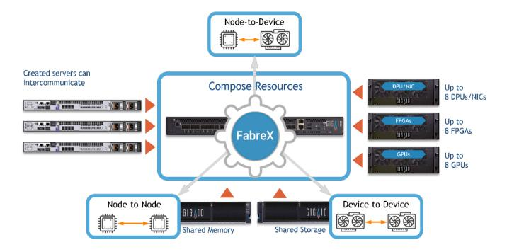
Communication between these resources consists of exclusively using the memory semantics of 'Memory Read' and 'Memory Write'. This means you can compose servers and CPUs in the exact same way as you compose end points (GPUs, FPGAs, ASICs, Smart NICs — anything with a PCle connection).
