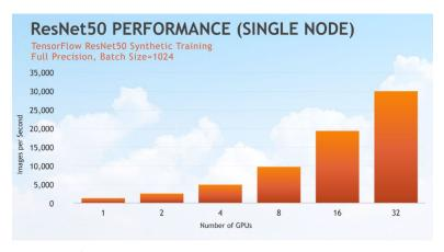
The **ResNet50** Performance graph (*above, at right*) shows the increase in images per second as GPUs are added to a SuperNODE.
